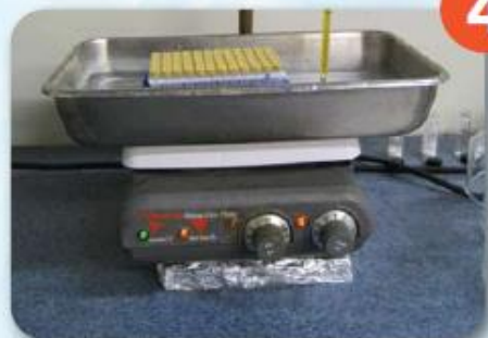
4 Heat the kit until vials contain homogeneous solution
