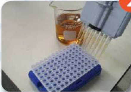
2 Add racemate and remove the "Transfer" solvent
