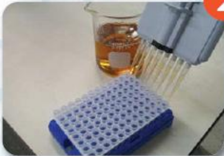
2 Add racemate and remove the "Transfer" solvent
