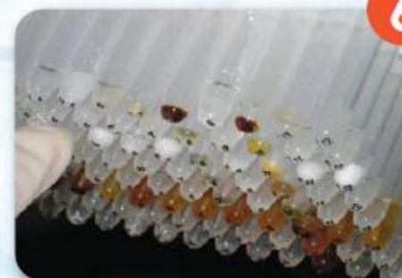
6 Identify vials with crystals for further analysis
